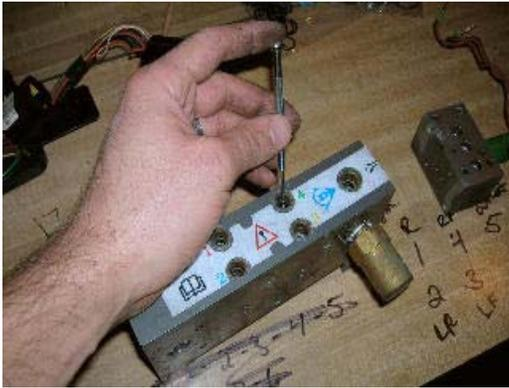
Remove the airline keepers with a large flat bladed screwdriver. Put under the lip and twist to remove.
