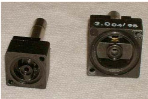
Disassemble the valve by removing the two remaining screws. The thinnest o-rings go over the valve stem, and seal it in the valve case. The old o-rings may be brittle as plastic because of age and pressure, yes you are looking at the right part. Re-assemble. Don't mix up the valve pieces, they are not interchangeable even though they look like they should be. Replace the 2 o-rings on the bottom of the valves (one small, one large).
