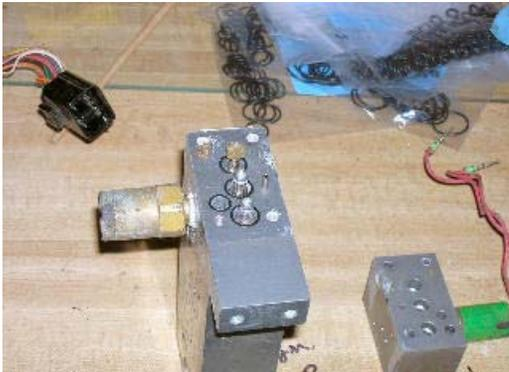
Replace the o-rings the reverse order they were removed. A little Vaseline will help seal and keep the o-rings in place.
