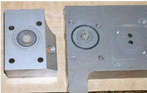
Remove the valves and the o-rings and set aside. (Keep the old o-rings just in case you lose or damage a new one.)
