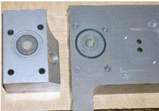
Replace the diaphragm and seal ring (same size as solenoid base rings) and diaphragm spring.
