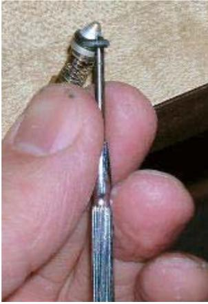
The trickiest part of the whole thing is removing the o-rings from the check valves. A small screwdriver pried underneath works fairly well, but be careful not to jab your fingers and don't damage the valve. You can also cut the o-ring with an Exacto knife if desperate, but I don't recommend it.
