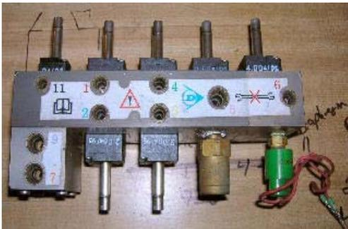
Replace the valves on the block, make sure you get them back in the original positions and don't pinch the o-rings. Valves 1-4 are interchangeable. If you forgot to mark them, the 4 with the smallest numbers (2.00 something) are 1-4 the middle number (2.5 something) is valve 5 and the largest (4.0) is valve 6. Valve 11 is small and only fits in one spot. Replace the valve top o-rings and replace the solenoids in their proper positions.
