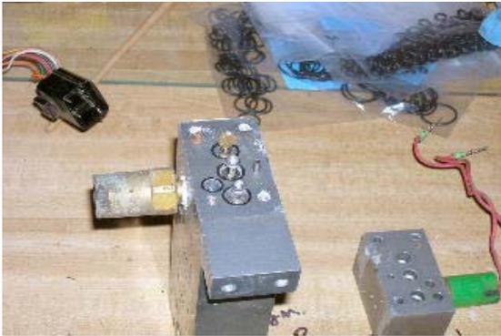
Remove the end block and the check valves.
