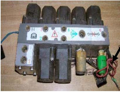
To remove the pressure switch wires from the driver multi-plug (the two red ones in the lower right corner of the picture, coming out of the green pressure switch) remove the yellow cover inside the plug and with a small screwdriver, release the catch on the pin, and pull the wire out the back of the plug. (easier said than done) it doesn't matter which way they go back in. Remove the block driver from the block and you're ready to disassemble.
