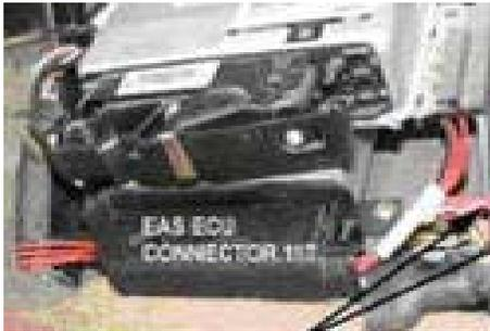
First **de-pressurize the system and springs**. With the engine off, disconnect the EAS ECU, under the drivers seat, bolted to the floor. If you unplug with the key "on" you'll hard fault the ECU and have to go to the dealer for a reset. Pin 1 has power for appx 1 minute after opening the door, so after you have the jumpers hooked up, put the key in and turn to position II for constant power. Turn the radio and A/C off so you can hear the compressor run, and the solenoids clicking.
